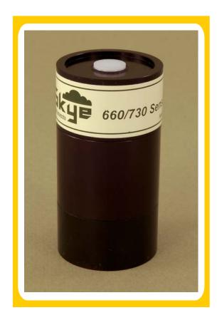
The sensor is a 2 channel radiometer, essentially two sensors in one. The specially designed light collecting head (fully Cosine Corrected) randomly splits light between two separately filtered photodiodes, giving a light intensity output for each of the red and far-red channels, ideal for measuring the RFR Ratio.
